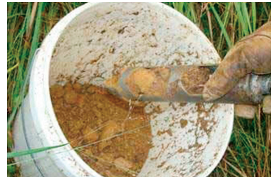
Thoroughly mix soil cores in a bucket to produce a more representative sample.
